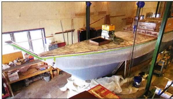
Sirens Boatworks of Merrickville, Ontario, is restoring a 38' Tiki catamaran built by her owner in the 1970s to a James Wharram design.
